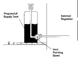
IMPORTANT: Install equipment shutoff valve in an accessible location. The equipment shutoff valve is for turning of or shutting off the gas to the appliance Apply pipe joint sealant lightly to male threads. This will prevent excess ant from going into pipe. Excess sealan in pipe could result in clogged heater valves.
